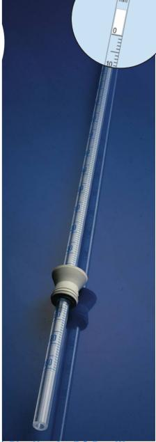
Pipettes for E.S.R. with zero levelling and automatic closure system for conventional tubes or AQUISEL Valve-Stopper.
