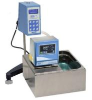
Immersion thermostat Digiterm controlling temperature of viscometer.
